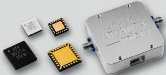
AM3025A – 7 Band Filter Bank in a 9mm QFN
